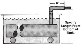
**XS76:** Straight thread with nut. Specify thread size and if bushing is to be standard (hex outside vessel) or inverted (hex inside vessel).
